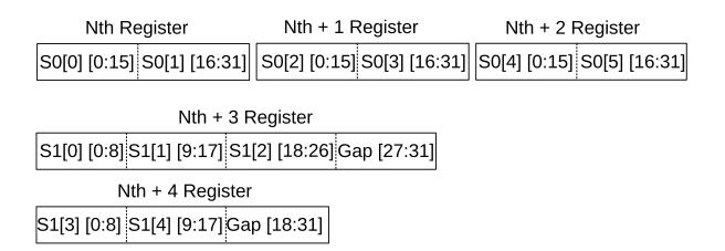
Figure 7.6: Example register layout of data of Array Multiple access type.
