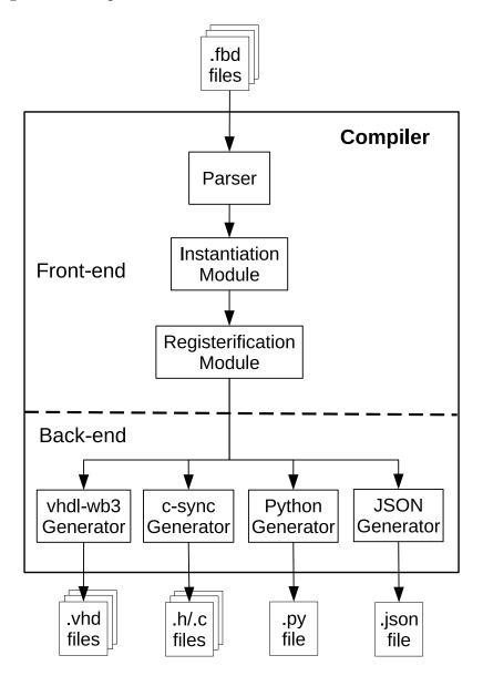
Figure 7.1: Current structure of the implemented compiler.
