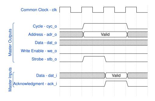
Figure 2.4: Wishbone classic standard single read transaction.
