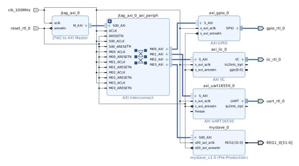
Figure 3.1: A simple design created using Block Designer in Xilinx Vivado environment [50].
