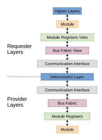
Figure 1.2: Conceptual stack of layers in the register-centric approach.
