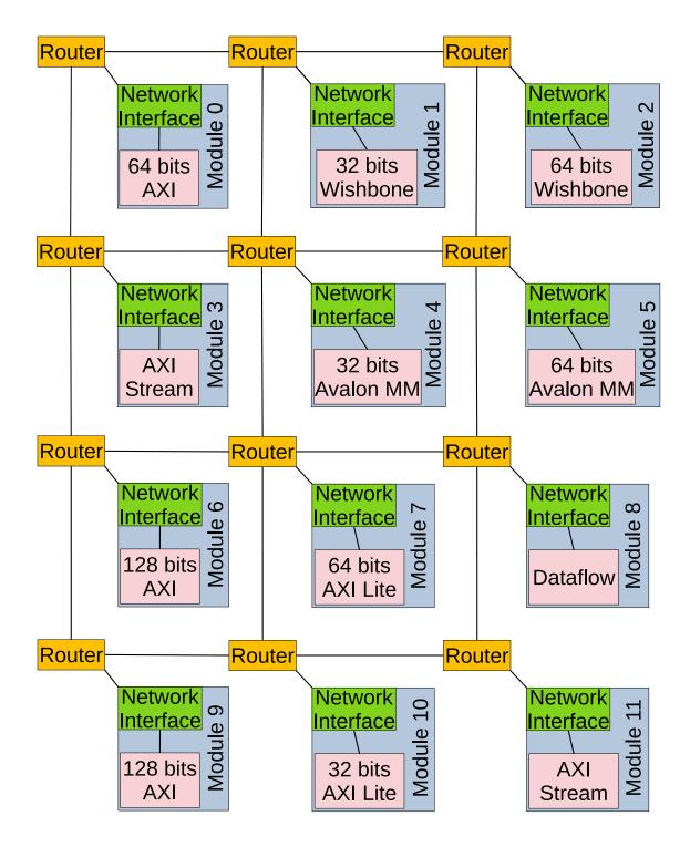
Figure 2.5: Example 12 nodes mesh network on chip.
