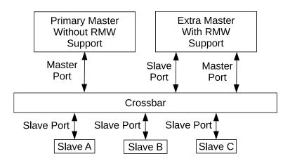
Figure 7.13: Example bus structure with extra master providing **rmw** transaction support.
