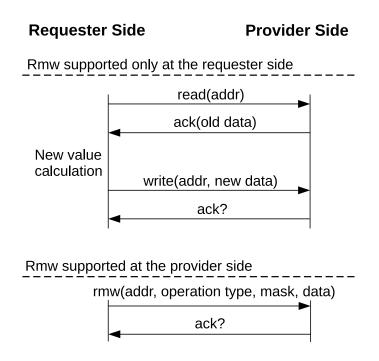
Figure 7.12: Sequence diagrams for **rmw** transaction without and with provider support for **rmw**.
