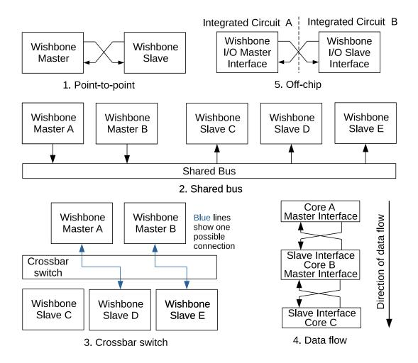
Figure 2.3: Possible Wishbone interconnections.
