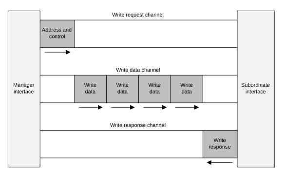
Figure 2.1: AXI channel architecture of writes [4].
