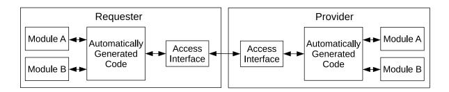
Figure 7.11: Simplified connection scheme of a system utilizing FBDL.
