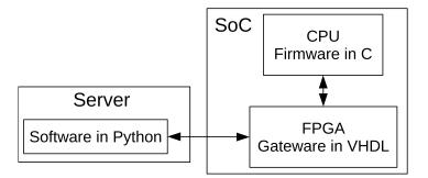
Figure 6.1: Example system with enumeration types synchronization issue.
